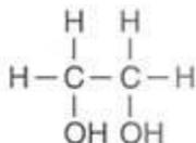
At standard atmospheric pressure, the boiling point of ethylene glycol is 198°C, compared to ethene that boils at -104°C.
